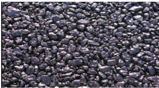
Gambar 1. Permukaan Aspal Porous (*UNHSC Design Specifications For Porous Asphalt Pavement and Infiltration Beds)
